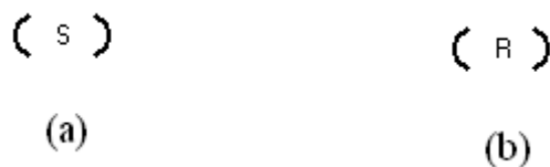
Figure 3.5: (a) Ladder Symbol for Set Coil (b) Ladder Symbol for Reset Coil
