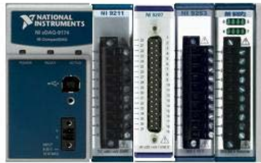
Figure 4.4: cDAQ & Its Modules
