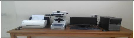
Device name: Vickers hardness tester
