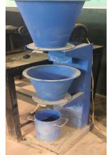
**Device Name: Compacting Factor Apparatus**
