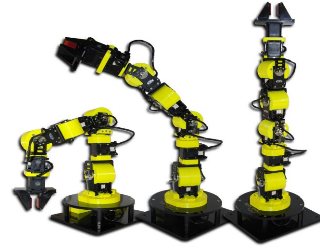
7DOF CYTON EPSILON 1500 Robotic Arm Manipulator
